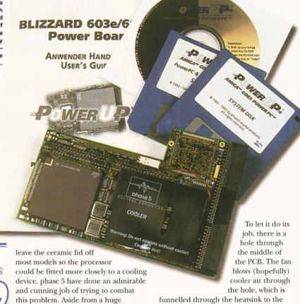
of the board, there is also a cooling fan. However, due to height restrictions, the fan has to be unconventionally situated on the underside of the board.
